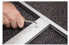
**STEP 2: (FOR 30 X 50 FRAME ONLY)** Insert the cross brace into the slots in the middle of the 50" side. Tighten the connection using the cross brace wrench.
