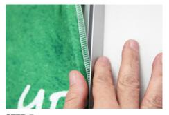
**STEP 5:** Continue pushing the silicone strip along the frame. The fabric will stretch to fit the frame without any wrinkles.
