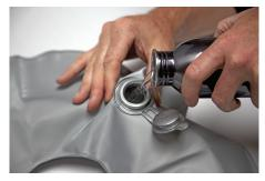
**STEP 2:**Open fill plug on the round water bag and fill with water or sand.
