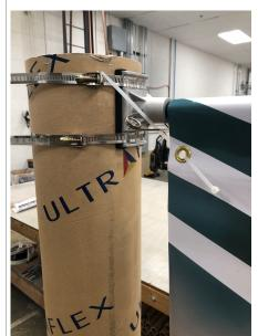
**STEP 2:** Secure base & pole assembly to light pole with two metal straps at appropriate height for top of light pole banner.
