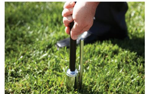
Slide the largest diameter rigid pole onto the ground spike's swivel post
